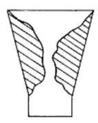
Figure 2.15 Bridging (left) and rat holing (right)
