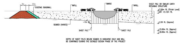
Figure 2.23 Barge unloading facility typical section
