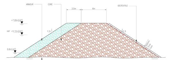
Figure 2.20 Western Basin Expansion typical section of peripheral bund wall – armour, core and geotextile (bund wall type B1)
