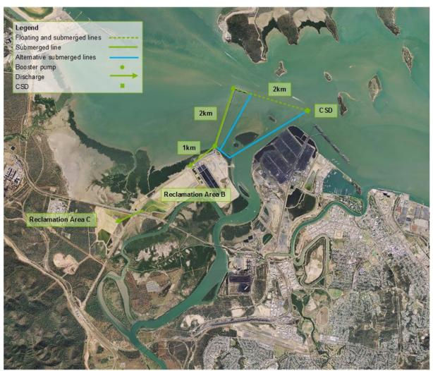
Figure 2.7 Wiggins Island Coal Terminal Project dredging and reclamation infrastructure placement arrangement
