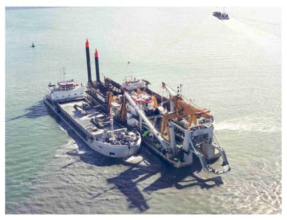
Photograph 2.6 Large cutter suction dredger loading barge
