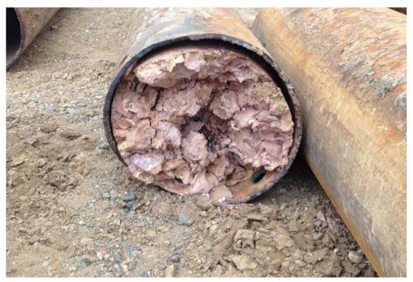
Photograph 2.3 Submerged pipeline blockage during the Western Basin Dredging and Disposal Project dredging (diameter of pipeline is 900mm)
