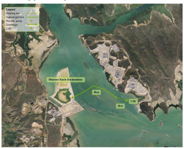
Figure 2.8 Western Basin Dredging and Disposal Project dredging and intertidal reclamation arrangement
