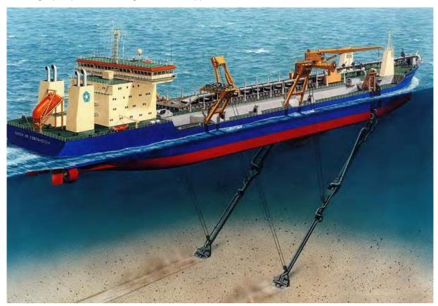
Figure 2.13 Typical trailing suction hopper dredger
