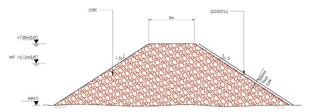
Figure 2.21 Western Basin Expansion typical section of bund wall – core material and geotextile (bund wall type B2)
